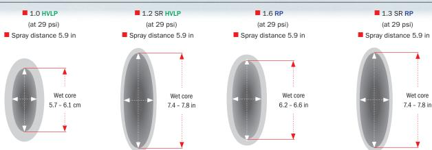
Standard nozzles with wet, compact core. SR nozzles with wide-stretched core.
