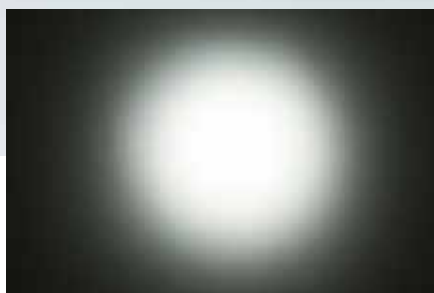
Example daylight lamp manufacturer C inconsistently illuminated surface, edges appear greenish/bluish
