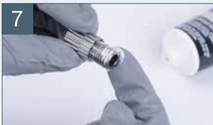
Lubricate* thread of material flow control screw
