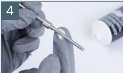
Lubricate* paint needle around the needle packing area
