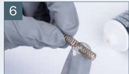
Lubricate* and insert paint needle spring
