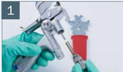
1 Removing the paint needle
