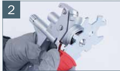
Hand-tighten fluid tip with universal spanner
