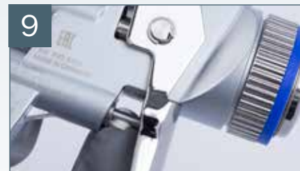
Lubricate visible area of air piston rod
