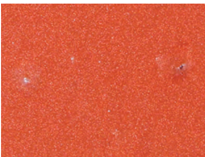
Dust particle inclusions
