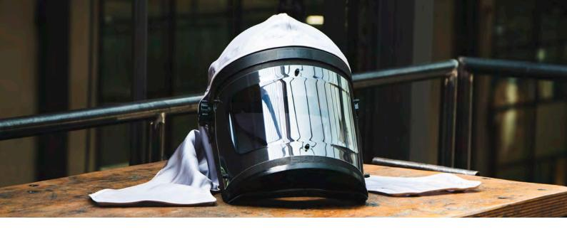
The SATA vision 2000 offers maximum protection when processing paint materials. The lightweight hood with the simple belt system allows fatigue-free working without endangering the health of the painters. In combination with the optional air warmer or cooler, the air temperature can be adjusted individually.
