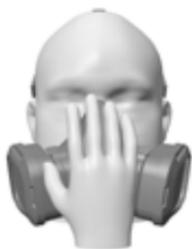
2. Breathe out normally. A correct seal is achieved when the mask body lifts slightly without causing any leakage between the mask body and the face.
