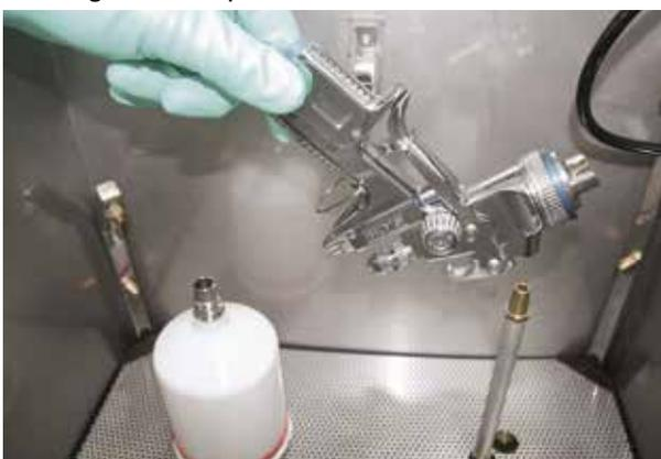
2. Connect air connection to air inlet
