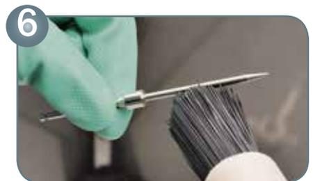
When cleaning the nozzle components, please make sure that metal parts of brushes do not damage the nozzle set. Ideally, please use specially designed SATA cleaning brushes and SATA nozzle cleaning needles to ensure optimum cleaning and maintenance of the nozzle set.
