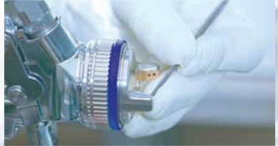
**Hand adjustment:** Each nozzle set is separately manually "tuned" to optimise the spray fan.
