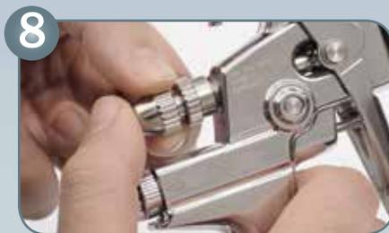
Install material flow control screw
