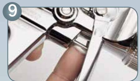
Grease visible part of air piston rod
