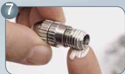
Grease thread of material flow control screw
