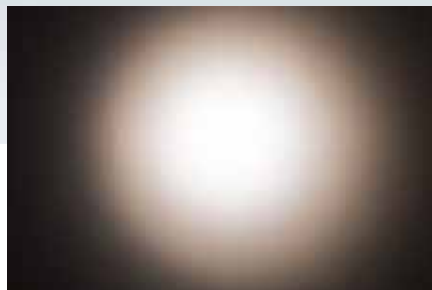
Example daylight lamp manufacturer D inconsistently illuminated surface, edge appear reddish.
