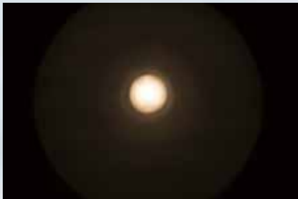
Example high quality torch manufacturer A Very small, non-uniformly illuminated surface, strong yellow coloration
