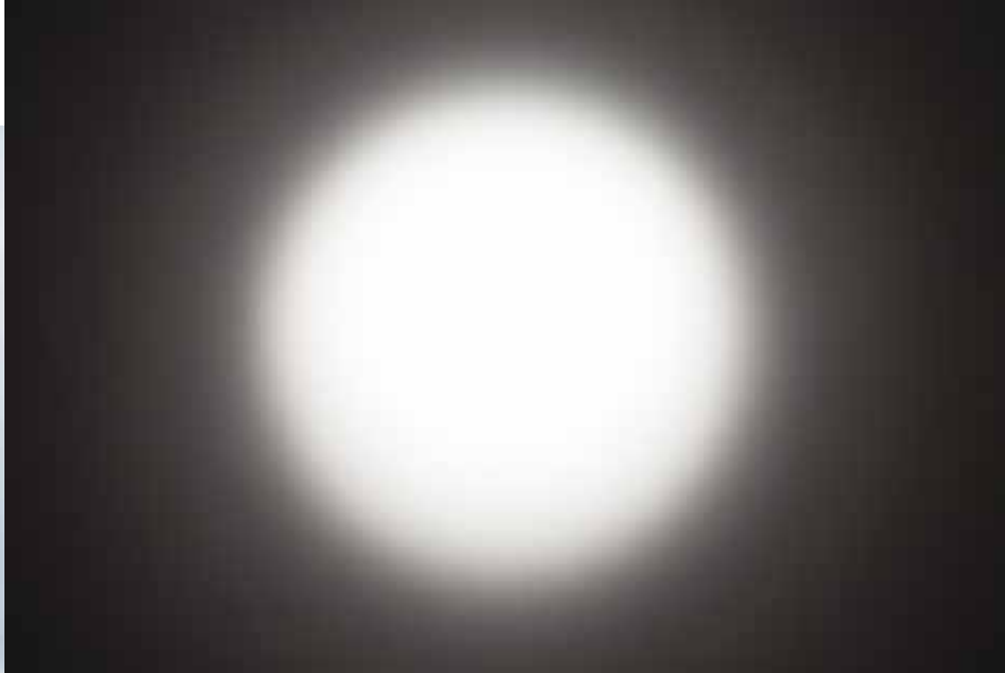
Light cone of the SATA trueSun at maximum light power, uniform distribution of the light intensity – colour temperature neutral
