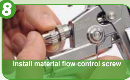
Grease thread of material flow control screw
